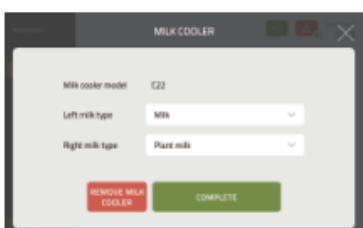
10. Enter the coffee machine menu, select System-Accessory-Milk cooler and install the milk cooler according to the instructions
